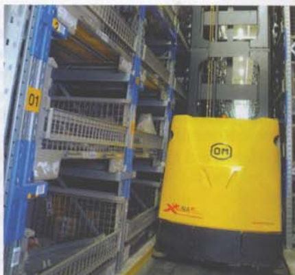
The reach truck has a three point layout structure - two load wheels and one drive wheel and stability pads under the driving cab.
